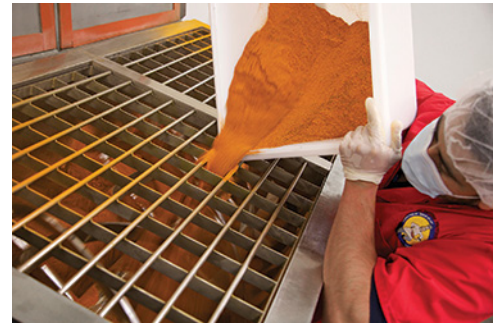
Operator weighs, measures, and loads individual spices into the Munson HE-2-1/2-5-SS ribbon blender to create one of Al Dentes' many custom seasoning blends.
