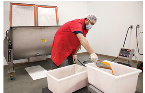
The ribbon blender's split double helical agitator, with 2:1 length-to-diameter ratio, promotes thorough mixing of ingredients. All surfaces contacting ingredients are constructed of #304 stainless steel.
