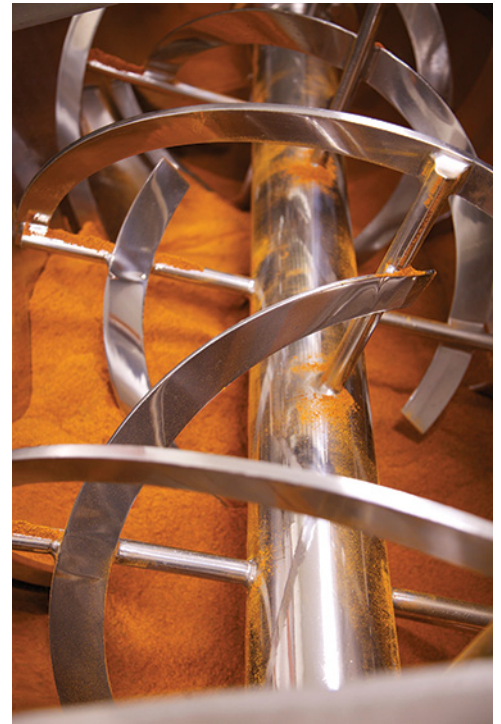
The ribbon blender's split double helical agitator, with 2:1 length-to-diameter ratio, promotes thorough mixing of ingredients. All surfaces contacting ingredients are constructed of #304 stainless steel.
